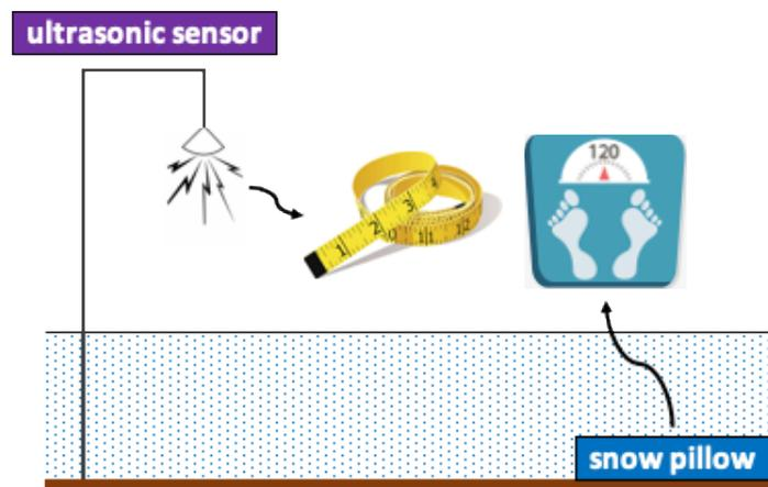
Snow telemetry (SNOTEL) stations are a great option. They measure the depth ( $H_s$ ) and the weight of the snowpack, which are used to calculate SWE. There are about 800 of these stations operating continuously in the western USA.
