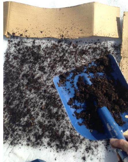
The cardboard was a simple but critical component that created the square shape and well-defined snow/sand border that later helped capture the students' attention visually. We used a probe to measure the snowpack depth in the center of each of the three plots (sand, control and duff) and took notes in order to make accurate comparisons later.
